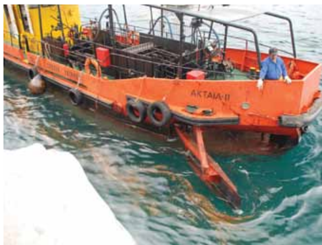
▲ Figure 1: A self-propelled weir skimmer for use in ports and nearshore waters. The bow doors open to enhance the swath and allow entry of floating oil. Recovered oil is pumped to an internal storage tank.
