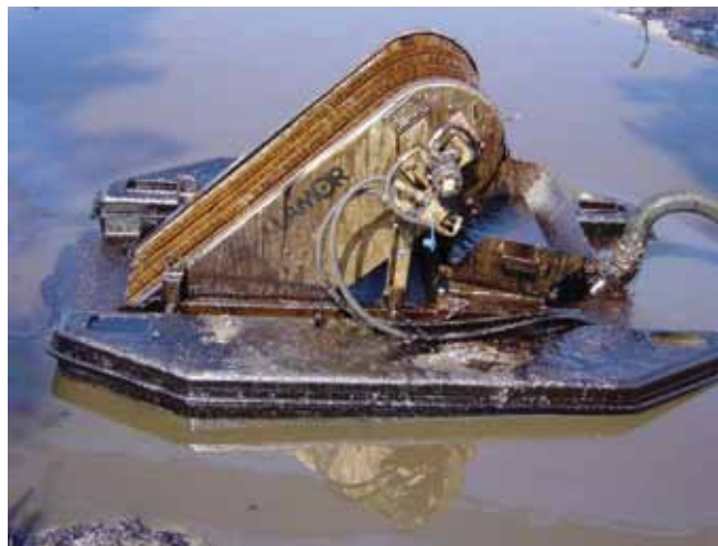
▲ Figure 5: Free floating brush skimmer. Oil adheres to the rotating brush sets and is lifted from the water surface. A comb removes the oil from the brushes to storage. A propeller behind the brush draws floating oil towards the skimmer to enhance the encounter rate and throughput (Image courtesy Lamor).
