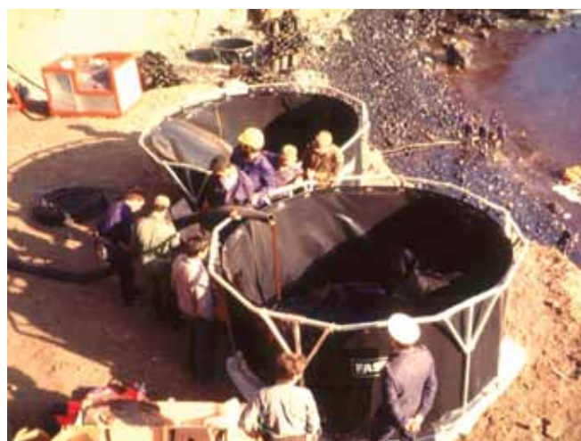
▲ Figure 28: Emulsified fuel oil recovered from the shoreline by skimmers and pumps into temporary storage tanks placed at the top of a cliff.
