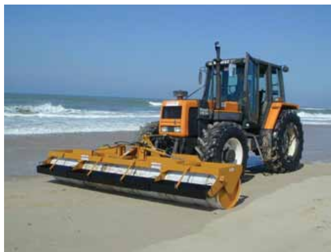
▲ Figure 36: Tractor-mounted oleophilic drum skimmer, used to collect fresh tarballs on a hard-packed sand beach (Image courtesy Le Floch Dépollution).
