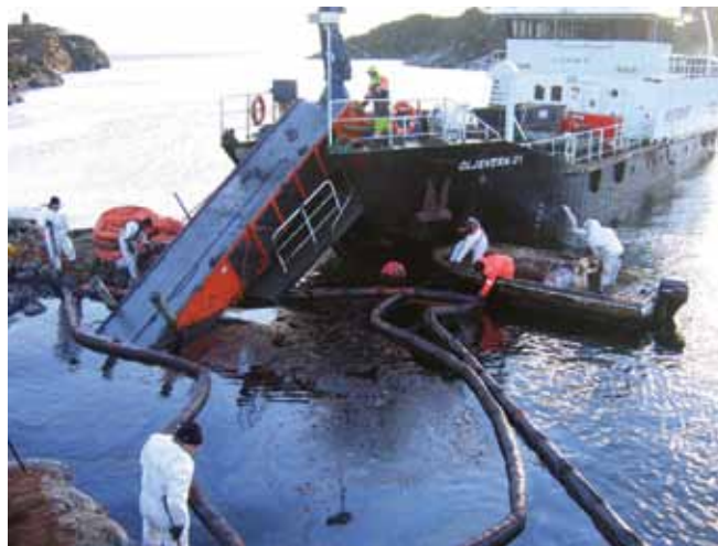
▲ Figure 15: A belt skimmer on a large recovery vessel. The belt, constructed from a mesh, allows water to drain through and encourages adhesion of the oil. The oil is lifted on-board and is scraped off to storage.
