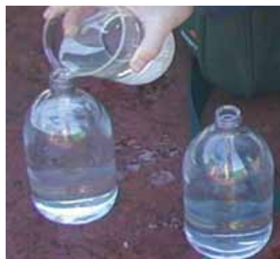
▲ Figure 12: Clear, narrow-mouth bottles (left) or plastic bottles (right) are not ideal containers for monitoring purposes.
