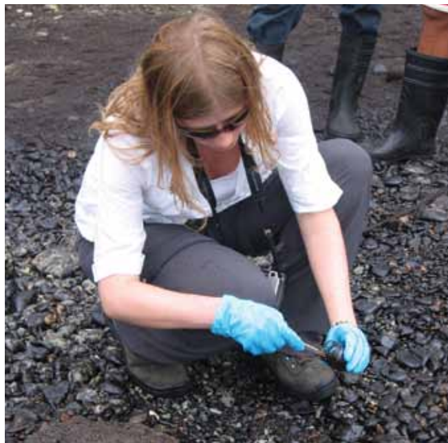
▲ Figure 7: Sampling stranded oil on the shoreline.
