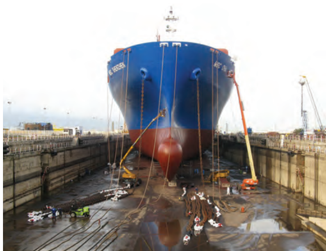
▲ Figure 6: Oil spills in dry docks can occur during routine maintenance operations.
